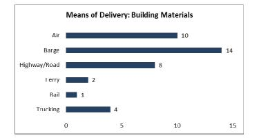
While these statistics do not necessarily discourage or promote prototype design, they suggest limitations on materials and products utilized. In general, the most limiting factors of air and water travel are weight and size of materials to be transported. Designs then must be limited to what can be effectively and efficiently transported by air and barge.
